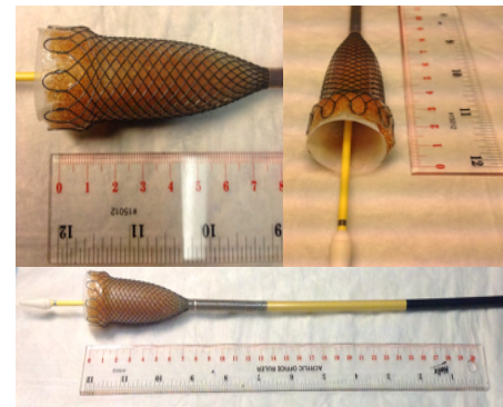
Fig 2. Prototype temporary catheter-based venous filter device. Boston-Scientific Wallflex stent is adapted with resin material (orange) sandwiched between two 200-micron mesh filters
