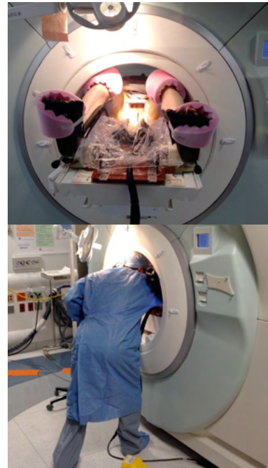
Figure 1. (A) The manipulator was docked on the patient table. (B) The needle was manually inserted by the radiologist in the 3T MRI scanner.
