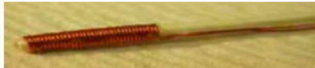
Figure 1. Solenoidal coil-tipped catheter, 30 AWG copper wire
